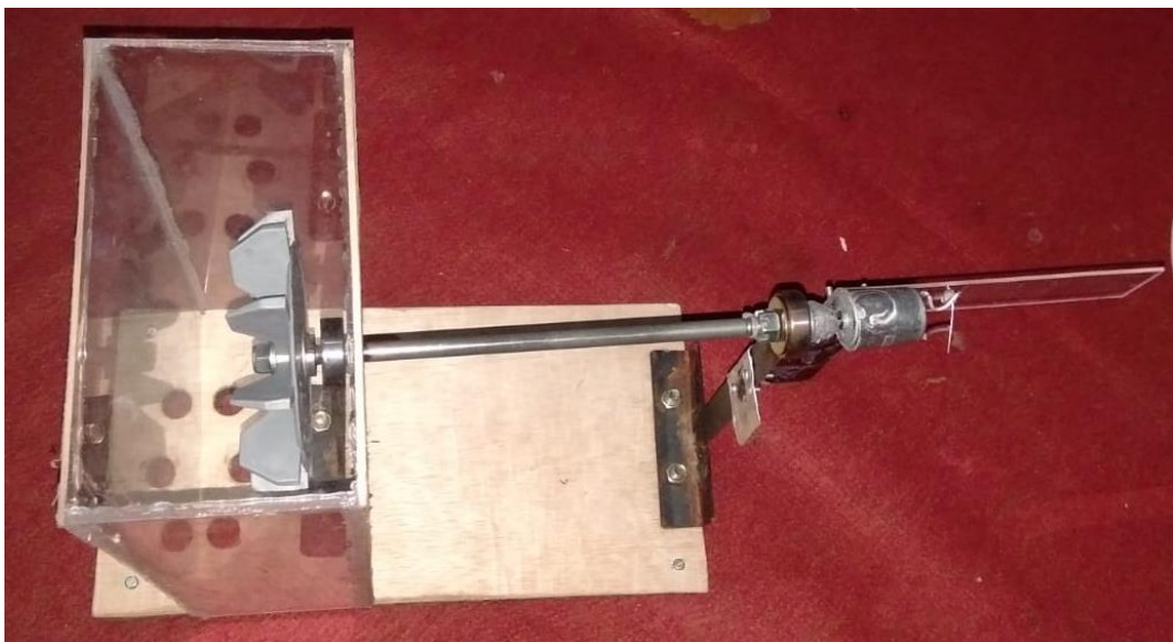
Figure 2. Set of micro-hydro power generation media
